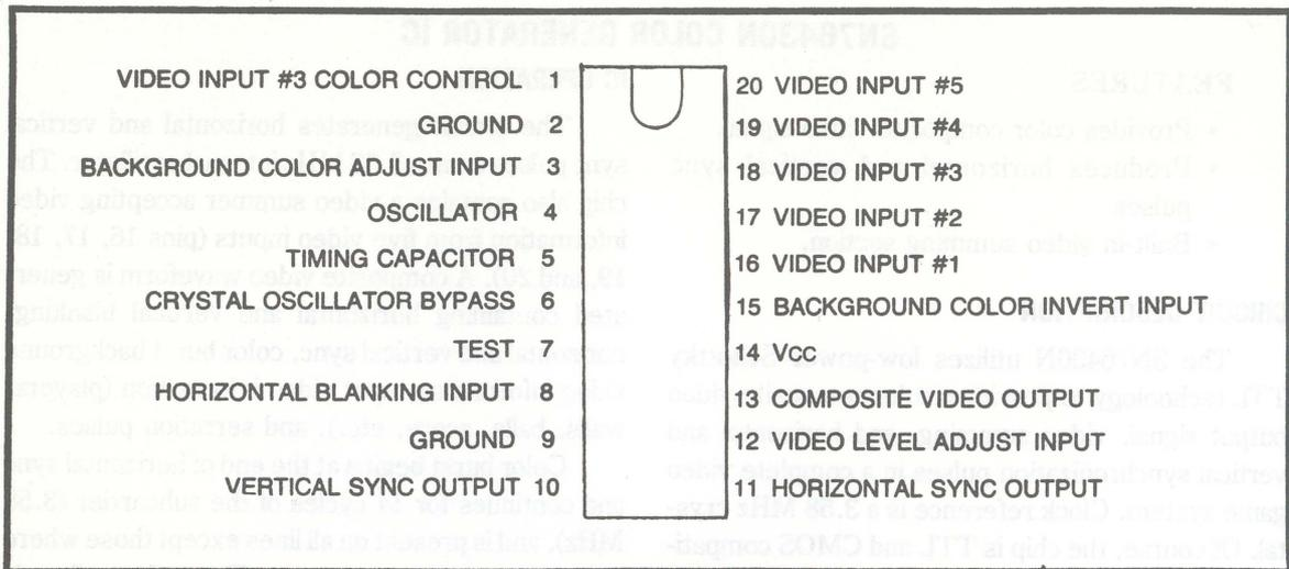
Fig. 6-15. SN76430N IC pin assignment.
