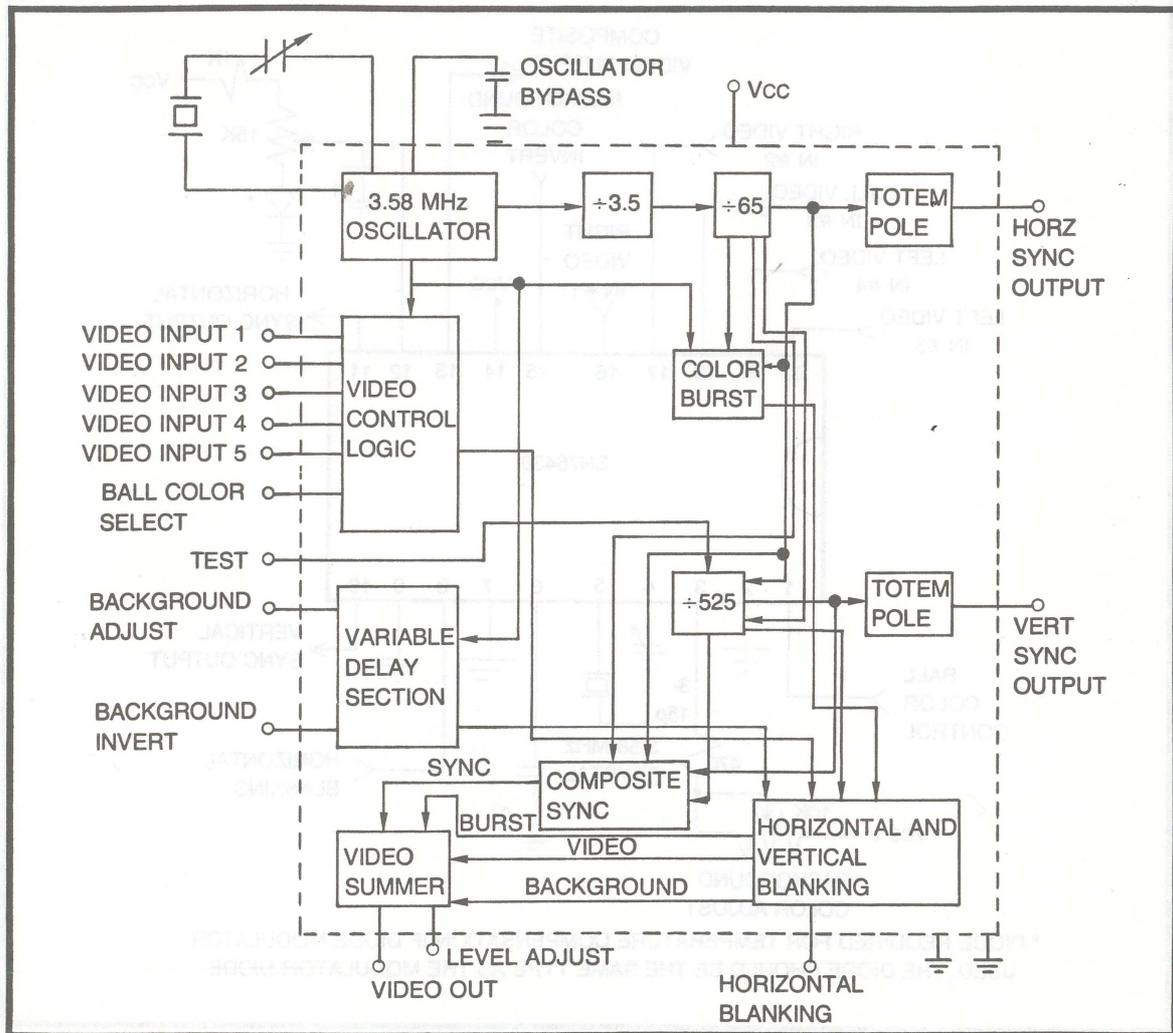
Fig. 6-14. Block diagram for the SN76430N IC.
