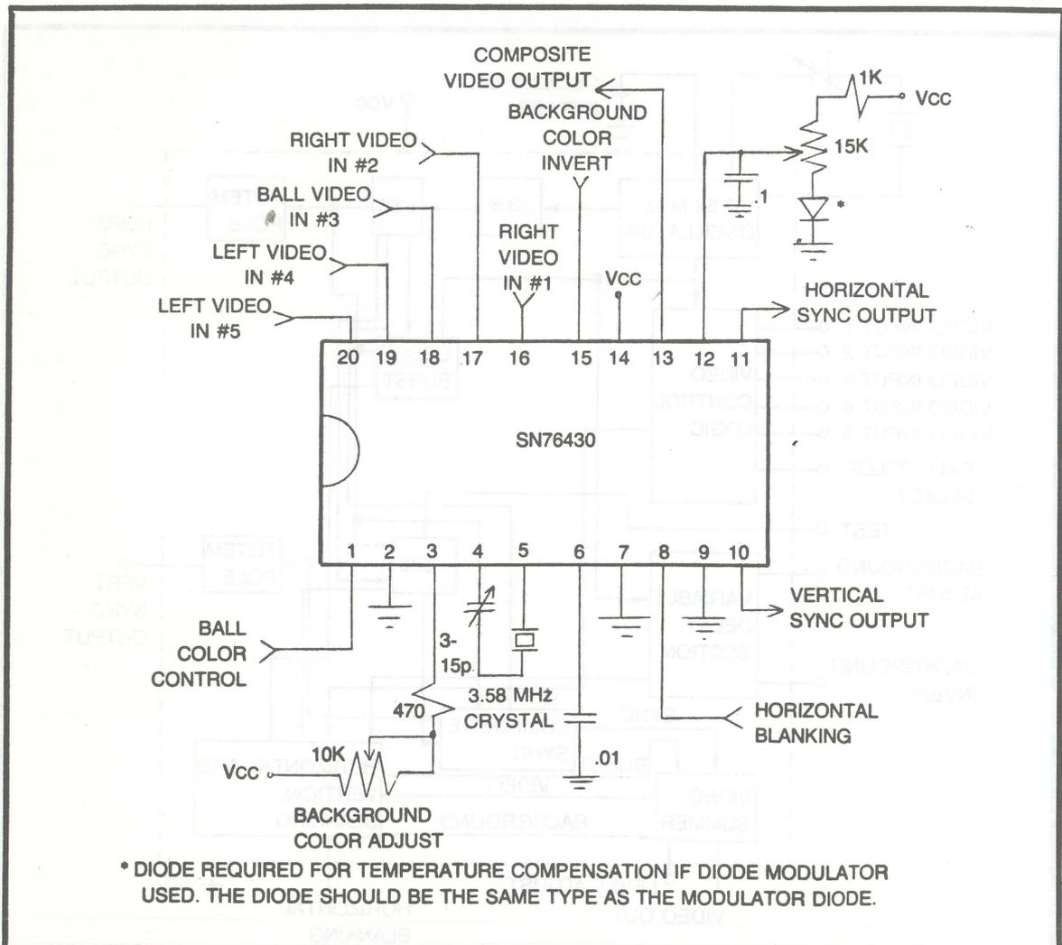
Fig. 6-16. Application schematic of the SN76430.
