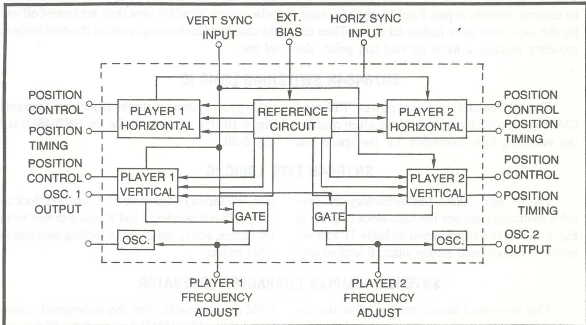
Fig. 6-17. Block diagram of the SN76431N IC.
